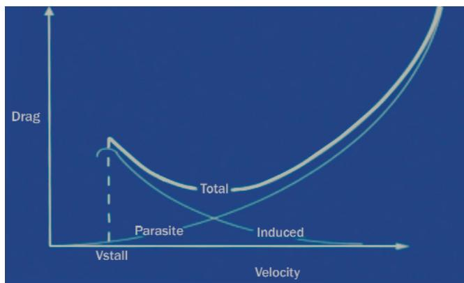
Figure 2: Indicated airspeed vs drag.
